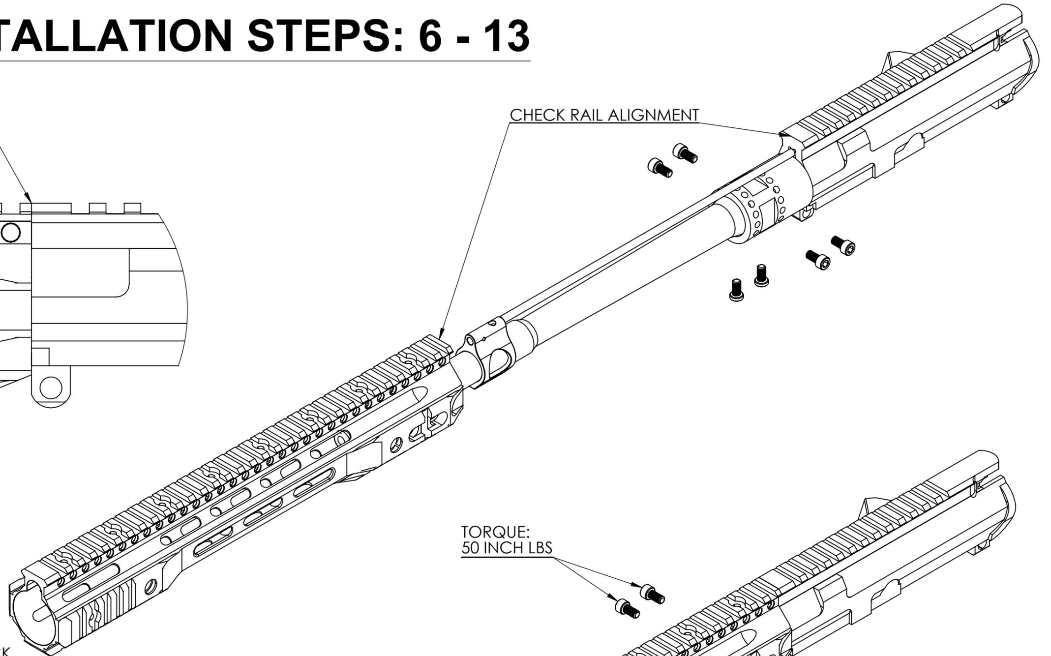
INSTALL LOW PROFILE GAS BLOCK AND GAS TUBE AFTER BARREL NUT IS INSTALLED
