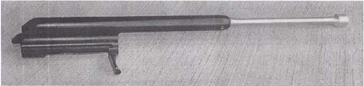
Bolt carrier with pinned arm or piston
